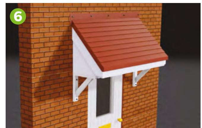
6 The Gallows Brackets are fixed to the canopy soffit in two places on each bracket. The Gallows Brackets are NOT to be used as the main structural support for the canopy. The upstand must be over flashed in lead or mastic sealed.
