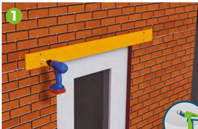
1 Position template central to the opening at the desired height. Using the centre of the 3 holes drill hole for fixing. Fix one side of template to wall, level up and repeat for other side of template.
