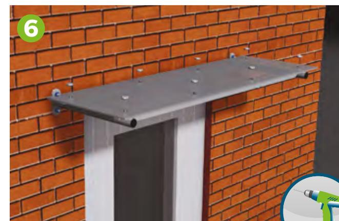
6 Place remaining threaded glass clamps and rubber washer seals on top of polycarbonate sheet. Remove the film from the top of the polycarbonate sheet. Working from the centre outwards loosely tighten the glass clamps onto the pole studs. Fully tighten the pole fixings and then all the glass clamps.
