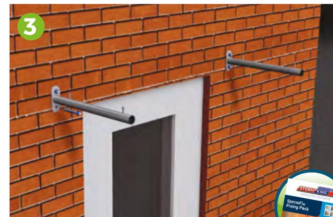
3 Loosely secure poles to wall in pre-drilled holes, with StormFix 80 Fixing provided. Place plastic end caps to support poles. Lay cross bars onto support poles with vertical section of bar facing front.
